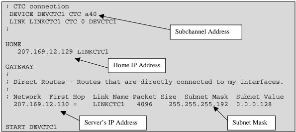
Figure 6-6. Mainframe TCP/IP Profile
